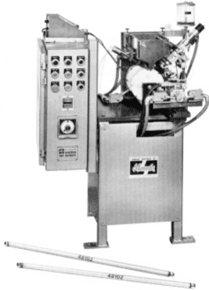
Vertical Automatic for marking Automotive push rods, tubing punches, etc . 1800 P .PH.
